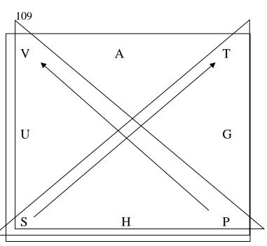
Once again the direction of the arrow gives the direction for each term. Since both arrows go up both terms are positive. So the Maxwell relation for this side is  $(\partial V/\partial S)_p = (\partial T/\partial p)_S$ . To find other Maxwell relations just turn the square on its side.
